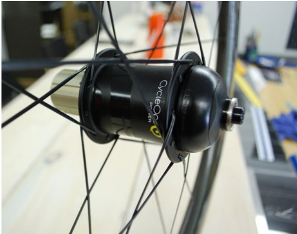
Fig. 1 A CycleOps PowerTap power meter (“Zipp 404 Firecrest Powertap G3 Wheel,” © Glory Cycles, used under Creative Commons Attribution license, http://creativecommons.org/licenses/by/2.0/ ) in a bicycle wheel hub. Data are transmitted wirelessly to a bicycle computer
