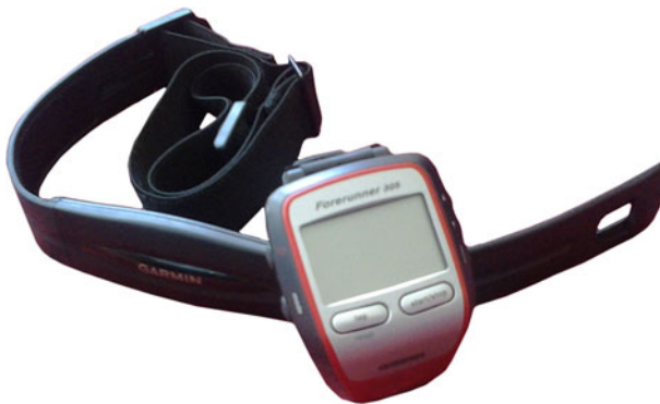
Fig. 2 Garmin Forerunner 305. The device is a GPS wristwatch that wirelessly communicates with a heart rate monitor. Additional sensors can be paired as well
