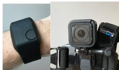
Fig. 1. The Empatica E4 device (left) that continuously tracks EDA and the wearable GoPro Session camera that records video.
