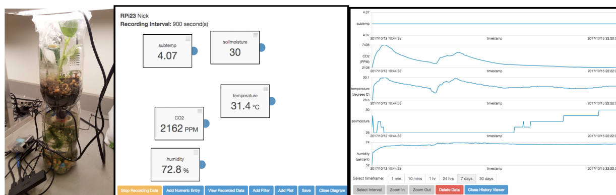
Figure 3. A student data-collection setup using networked sensors and the Dataflow tool developed by Concord Consortium (image courtesy of Sherry Hsi)
